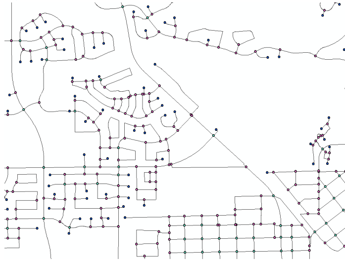
Figure 4.6 Street Intersection [NODE] Layer
